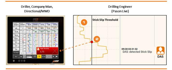
DAS Stick-Slip will show the estimate of downhole stick-slip calculated by the model. The values mean the following:
